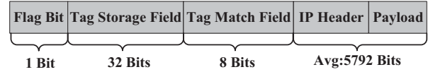
Fig. 4: Tag Storage/Match Fields and Flag Bit in a packet. Flag Bit Field indicates whether the packet has been embedded a tag or not. Tag Match Field stores the first NF in the SFC and Tag Storage Field embeds the rest NF(s) in the SFC. The overall bandwidth cost for embedding tags is negligible.
